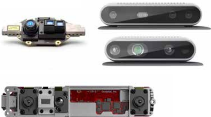
Figure 5. The latest generation of small, low-cost, and low-power 3D cameras enable robust vision deployments (above); their infrared illumination modules are similarly becoming increasingly cost-effective (below).
