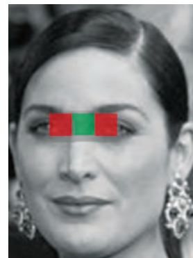
A Haar feature consists of multiple adjacent areas that are subtracted from each other. The Viola - Jones approach suggests recommends Haar features containing 2, 3 and 4 areas. The encoding signature = Pixels under Green - pixels under red.
